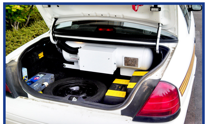
The autogas tank inside a Crown Victoria
